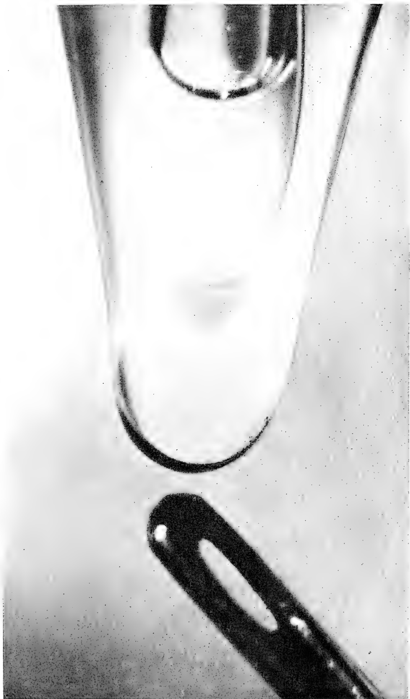
PRECIPITATE OF AMERICIUM HYDROXIDE IN CAPILLARY TUBE Eye of needle shows degree of magnification.
